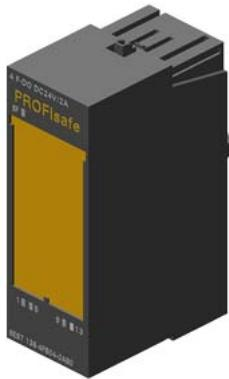
SIMATIC DP, Electronics module for ET 200S, 4 F-DO PROFIsafe, 24 V DC/2 A, 30 mm overall width, up to PL E (ISO 13849), up to SIL 3 (IEC 61508), can also be used in PROFINET configuration with IM 151-3 HF
