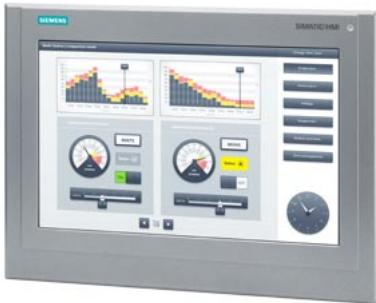
SIMATIC HMI TP1500 Comfort Outdoor, Comfort Panel, Touch operation, 15" widescreen TFT display, 16 million colors, PROFINET interface, MPI/PROFIBUS DP interface, 12 MB configuration memory, Windows CE 6.0 (Microsoft Support included Security updates discontinued) configurable from WinCC Comfort V13 SP1, HSP
