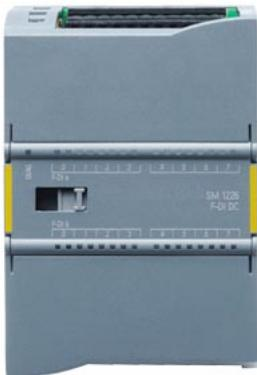
SIPLUS S7-1200 SM 1226 F-DI 16x24VDC based on 6ES7226-6BA32-0XB0 with conformal coating, -25...+55 °C, F-DI 16x 24 V DC, PROFIsafe, 70 mm width, up to PL e (ISO 13849-1)/ SIL3 (IEC 61508)
