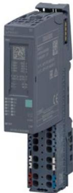
SIMATIC ET 200SP TM ECC 2xPWM ST Chargecontroller f. conductive charging of electric vehicles according IEC61851 mode 3 for 2 Charging points -30°C...60°C 2x Control Pilot 2x Plug Present 2x DQ switch contact for contactor; 2x DI read contact for contactor or connector locking; 2x ACT for connector locking suitable for BU Typ BU20-P12+A0+4B and BU20-P12+A4+0B
