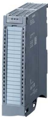
SIMATIC S7-1500, digital input module DI 16x 24...125 V UC HF, 16 channels in groups of 1; input delay 0.05..20 ms; Input type 3 (IEC 61131); Diagnostics, hardware interrupts: Front connector (screw terminals or push-in) to be ordered separately
