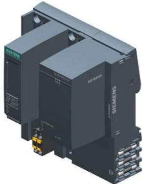
SIMATIC ET 200SP, PROFINET, 3-port interface module, IM 155-6PN/3 High Feature, 2 slots for BusAdapter, max. 64 I/O modules and 16 ET 200AL modules, S2 redundancy, multi-hotswap, 0.25 ms, isochronous mode, optional PN strain relief, including server module
