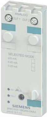
SIPLUS AS Interface 2 AQ IP67 based on 3RK1107-1BQ40-0AA3 with conformal coating, -25...+70 °C, AS-Interface compact module, IP67 analog, 2 AQ, number format S7, 2x 1 output (M12), 4...20 mA for 2-wire actuators . mounting plate 3RK1901-0CA00 must be ordered separately
