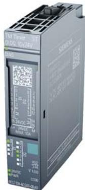
SIPLUS ET 200SP TM timer DIDQ 10x24V based on 6ES7138-6CG00-0BA0 with conformal coating, -40...+60 °C, time-controlled digital inputs and outputs 4 DI, 6 DQ with time stamp count, PWM, oversampling
