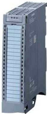
SIMATIC S7-1500, digital output module DQ16x24..48VUC/125V DC/0.5A ST; 16 channels in groups of 1; 0.5 A per group; substitute value: observe derating the module supports the safety-oriented shutdown of load groups up to SIL2 according to EN IEC 62061:2021 and Category 3 / PL d according to EN ISO 13849-1:2015. front connector (screw terminals or push-in) to be ordered separately
