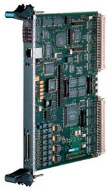
SIMATIC TDC Communication module CP 52M0 Memory module for Global Data Memory (GDM) with 2 MB SRAM memory
