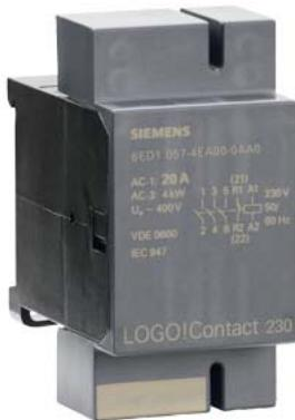
LOGO! contact 230 Switching module for direct switching of resistive loads up to 20 A and motors up to 4 kW, 230 V AC, 3 NO contacts+1 NC EAN: 4025515050759
