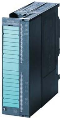
SIPLUS S7-300 FM350-1 based on 6ES7350-1AH03-0AE0 with conformal coating, -25...+60 °C, counter module counter functions up to 500 kHz 1 channel for connection of 5 V and 24 V incremental encoders isochronous mode; measuring range types incl. configuration package on CD-ROM
