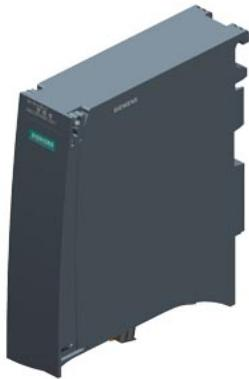
SIPLUS ET 200MP IM155-5 PN ST TX rail based on 6ES7155-5AA01-0AB0 with conformal coating, -40...+70 °C, OT4 with ST1/2 (+85 °C for 10 minutes), PROFINET IO device interface module for ET 200MP electronic modules; up to 12 IO modules without PS; up to 30 IO modules with additional PS; integrated 2-port switch; RJ45 shared device; MRP; IRT >=0.25 ms; isochronous mode FW update; I&M0...3; with 500 ms
