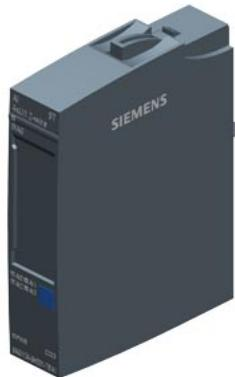
SIPLUS ET 200SP AI 4xU/I 2-w ST based on 6ES7134-6HD01-0BA1 with conformal coating, -40...+70 °C, analog input module, suitable for BU type A0, A1, color code CC03, module diagnostics, 16 bit, +/-0.3%
