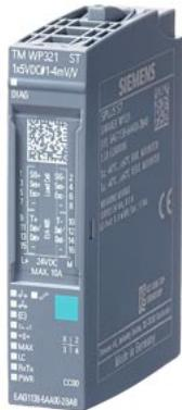
SIPLUS ET 200SP WP321 based on 7MH4138-6AA00-0BA0 with conformal coating, -40...+60 °C, electronic weighing system 1 channel for the connection of load cells DMS full bridges (1-4 mV/V) for SIMATIC ET200SP, suitable for BU type A0, RS485 interface for SIWATOOL or remote display.
