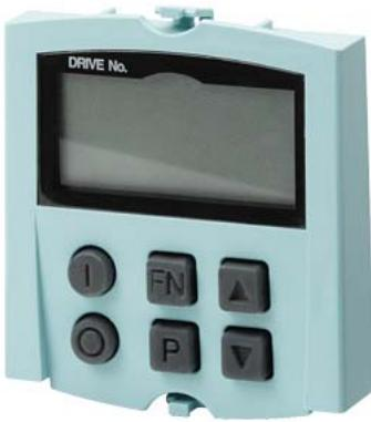
SIPLUS S120 BOP20 Basic Operator Panel based on 6SL3055-0AA00-4BA0 with conformal coating, -20...+50 °C, actuator with miniature display 2-line, 6 keys for parameter assignment and diagnostics suitable for Control Units CU305, CU310, CU320
