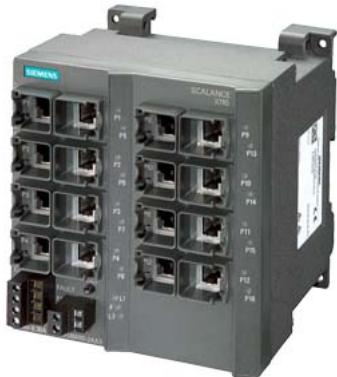
\*\*\*\*\* spare part \*\*\*\*\* SCALANCE X116, unmanaged IE switch, 16x 10/100 Mbit/s RJ45 ports, LED diagnostics, error-signaling contact with set pushbutton, redundant power supply manual available as a download .
