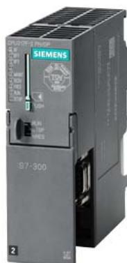
SIPLUS S7-300 CPU 317F-2PN/DP based on 6ES7317-2FK14-0AB0 with conformal coating, -25...+60 °C, central processing unit with 1.5 MB work memory, 1st interface MPI/DP 12 Mbps, 2nd interface Ethernet PROFINET, with 2-port switch, Micro Memory Card required
