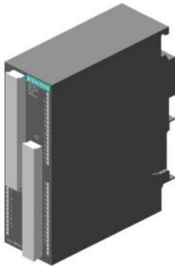
SIMATIC S7-300 digital output SM 322, Isolated in groups of 16, 64DO, 24 V DC, 0.3A sinking output Total current 2 A/group, 8 A/module Terminal blocks 6ES7392-1.N00-0AA0 and cable 6ES7392-4...-0AA0 required
