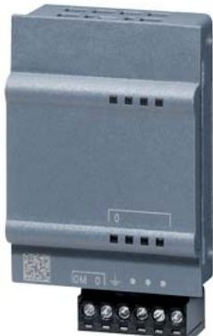
SIPLUS S7-1200 SB 1232 1AQ based on 6ES7232-4HA30-0XB0 with conformal coating, -20...+60 °C, analog output 1 AQ, +/-10 V DC (12 bit resolution) or 0-20 mA (11 bit resolution)
