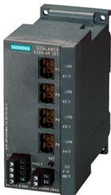
SCALANCE X200-4PIRT managed IE IRT switch, 4x 100 Mbit/s POF SC RJ ports, Error signaling contact with set pushbutton, Redundant power supply, PROFINET IO device, network management, Redundancy Manager integrated, incl. electron. manual on CD-ROM, C-plug optional.
