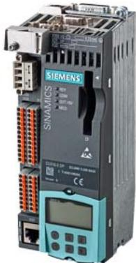
SIPLUS S120 Control Unit CU310-2 DP based on 6SL3040-1LA00-0AA0 with conformal coating, -20...+55 °C, with PROFIBUS interface without CompactFlash card
