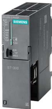
SIPLUS S7-300 CPU 315F-2PN/DP based on 6ES7315-2FJ14-0AB0 with conformal coating, -25...+60 °C, central processing unit with 512 KB work memory, 1st interface MPI/DP 12 Mbps, 2nd interface Ethernet PROFINET, with 2-port switch, Micro Memory Card required
