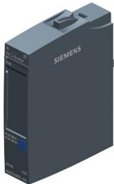
SIPLUS ET 200SP AI 4xI 2-/4-wire T1 rail based on 6ES7134-6GD01-0BA1 with conformal coating, -40...+60 °C, OT1 with ST1/2 (+70 °C für 10 minutes), analog input module, suitable for BU type A0, A1, color code CC03, module diagnostics, 16-bit, +/-0.3%
