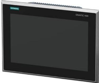
SIMATIC HMI TP1200 Comfort INOX Stainless steel front, Glass pane, capacitive touch, Degree of protection front IP69K, 12" widescreen TFT display, PROFINET interface, MPI/PROFIBUS DP interface, 12 MB configuration memory, Windows CE 6.0, (Microsoft Support included Security updates discontinued) configurable from WinCC Comfort V15
