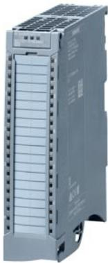
SIMATIC S7-1500 analog input module AI 8xU/R/RTD/TC HF, 16 bit resolution, up to 21 bit Resolution at RT and TC, accuracy 0.1%, 8 channels in groups of 1; common mode voltage: 30 V AC/60 V DC, Diagnostics; Hardware interrupts Scalable temperature measuring range, thermocouple type C, Calibrate in RUN; Delivery including infeed element, shield bracket and shield terminal: Front connector (screw terminals or push-in) to be ordered separately
