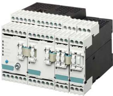
SIPLUS CMS2000 basic unit "VIB; 2 IEPE vibration channels; 2 analog inputs for "Process value; 1 digital input "for rotational speed acquisition;" System and limit value messages via 3 digital outputs
