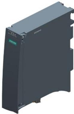
SIPLUS ET 200MP IM155-5 PN ST based on 6ES7155-5AA01-0AB0 with conformal coating, -40...+70 °C, PROFINET IO device interface module for ET 200MP electronic modules; up to 12 IO modules without PS; up to 30 IO modules with additional PS; integrated 2-port switch; RJ45 shared device; MRP; IRT >=0.25 ms; isochronous mode FW update; I&M0...3; with 500 ms
