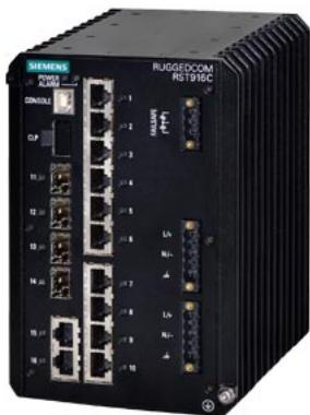
RUGGEDCOM RST916C is a 16 port industrially hardened, fully managed 10G Ethernet switch featuring integrated IEEE 1588 support for use in harsh industrial environments. The product has 4x 1/10Gbit/s SFP+ slots and 12x 10/100/1000Mbit/s RJ45 ports. -40°C to +85°C operating temperature (fanless).
