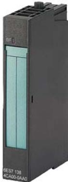
SIMATIC DP, Electronics module 2 AO I High Feature for ET 200S, 15 mm width, Cycle time per module: 0.5 ms, +/-20mA; 15 bit+sign, 4.. 20mA; 15 bits Operational limit +/-0.05% with SF LED (group fault)
