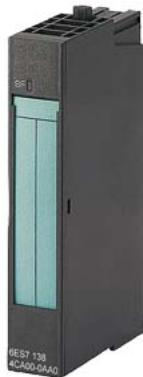
SIMATIC DP, Electronics module 2 AI U High Feature f. ET200S, 15 mm width, Cycle time per module: 0.5 ms, +/-10V; 15 bit+sign, +/-5 V; 15 bit+sign, 1.5 V; 15 bit, Operational limit +/-0.1% with SF LED (group fault)
