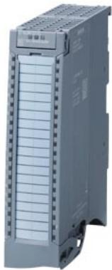
SIMATIC S7-1500, digital input module DI 16x24 V DC AUX; 16 channels in groups of 8; for 24 V encoder; sensor supply 24 V DC; input type 2 (IEC 61131); input delay parameterizable 0.05..20 ms; isochronous mode up to 250  $\mu$ s; integrated counting function up to 20 kHz; pulse stretching; chatter monitoring; signal inversion diagnostics; hardware interrupts: front connector (screw terminals or push-in) and, if applicable, order shield set separately
