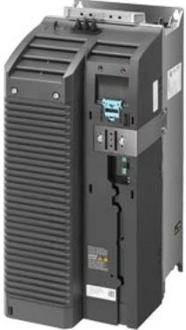
SIPLUS G120 PM240-2 IP20-FSD-A-400V 30 kW based on 6SL3210-1PE26-0AL0 with conformal coating, -20...+50 °C, with integrated class A filter with integrated braking chopper 380-480 V 3 AC +10/-20% 47-63 Hz power high overload: 22 kW at 200% 3 s, 150% 57 s, 100% 240 s power low overload: 30 kW at 150% 3 s, 110% 57 s, 100% 240 s 472x 200x 237 (HxWxD), design FSD, degree of protection IP20 without CU and operating unit released as of CU FW version V4.7 HF8
