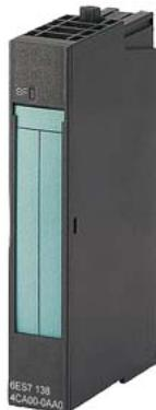
SIMATIC DP, Electronics module f. ET200S, 2AI Standard I-2DMU 15 mm width, 4..20mA; 13 bit for 2-wire transducer Cycle time 65 ms/channel with SF LED (group fault)
